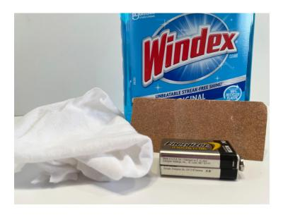
Wipe the bridgeplate clean with a clean cloth <u>lightly</u> moistened with water or Windex™, and allow it to dry for at least 10 minutes. NEVER use Naptha™, lighter fluid or any other cleaners like this to clean the bridgeplate or pickup, as these will leave deposits behind that will destroy any chance of obtaining a proper bond. Pure Acetone can be used to remove any stubborn adhesive left behind, but use it sparingly, and don't get it on the finish of your instrument.
