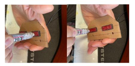
Once the pickups are placed on the bridgeplate, press each pickup against the bridgeplate with your fingers and wiggle it around a bit to make sure that the E6000 cement completely coats the area underneath the pickup. Using the mirror and light, make sure that the pickups are positioned correctly in the template, and that the template is sitting parallel to the bridgeplate so it doesn't stick to the adhesive.
