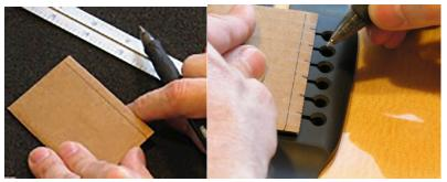
Using the ruler, draw a line about 1/4" inside along one edge. Then place the template centered next to the bridgepin holes. Mark the position of each of the holes along the edge of the template and on the line.
