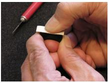
Apply a strip of the included temporary white adhesive to the red sensing surface of each of the pickups. Using your thumb, press the adhesive over the entire red sensing surface of the pickup to bond it.
