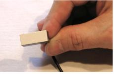
Trim the excess adhesive from the pickup on all sides, using a sharp pair of scissors, so you end up with the tape aligned with the edges of the pickups.
