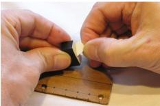
Remove the backing paper from the adhesive (an X-Acto blade can be helpful to help peel away the edge of the paper)
