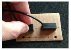
Place the pickups centered on the saddle line of the template in the positions shown. Weaken the stickiness of the adhesive first by pressing on it with your thumb for a while. The
