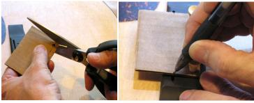
Remove the golf tees and place the template on a flat surface. Use a ruler to line up the two saddle slot marks on the template, and draw a line connecting them with a pen or pencil. You may want to create additional copies of your template including the marks for the location holes; if you decide to make adjustments later, this will give you a fresh blank to work from without having to recreate your work.
