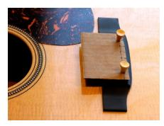
Carefully enlarge the holes to the proper size using the golf tees (or other), then place the template on the instrument bridge, putting the tees in the two outer holes to hold the template in place. Making sure that the template is parallel to the top of the guitar, mark the location of the saddle slot on each side of the template. If you can't see the saddle slot on each side, trim the width of the template so the saddle slot is just visible on each side so you can mark it.
