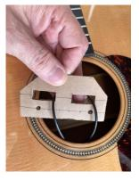
Once the adhesive is cured, carefully remove the template, sliding it up and over the pickups and golf tees, and sliding it along the wires to the soundhole. Using the scissors, cut the cardboard template tab between the
