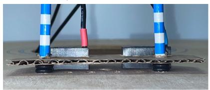
Then, using <u>light</u> finger pressure, hold the two pickups in place against the bridgeplate for 10 minutes. <u>Don't try to</u> force all of the adhesive out from underneath the pickups; you want to leave a thin layer of the adhesive between the pickup and bridgeplate as it cures.
