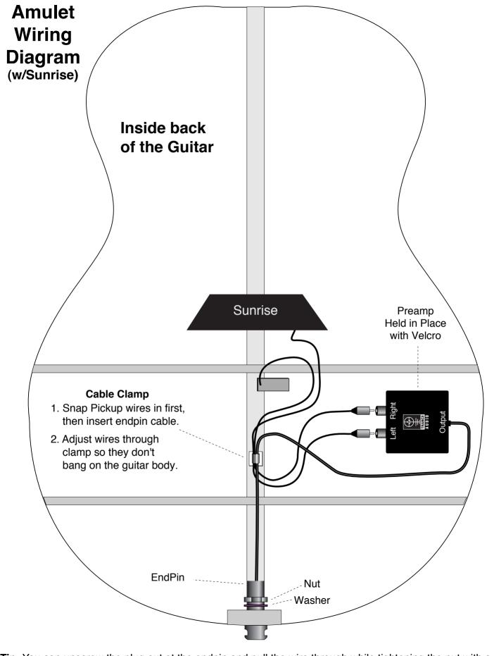
**Tip:** You can unscrew the plug out ot the endpin and pull the wire through while tightening the nut with a nutdriver. Then screw the plug back in using the plug on the guitar cord as a handle.
