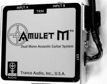
The clip on the side of the Amulet M preamp (adjacent to the EXT jack where the cable/battery clip plugs in) allows you to securely anchor the cable to the preamp and prevent it from being pulled loose or disconnected by vibration or cable routing problems.
