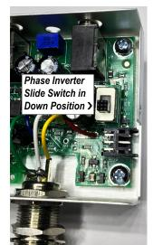
The **Phase Switch** is an internal slide switch that allows you to invert the phase of your signal, so you can perfectly match any additional pickups you might use with your instrument in a multi-system setup. This can also be used to help to increase gain before feedback in difficult monitoring situations.
