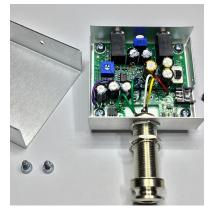
The **Amulet M Plus**™ has new features and to access these new features, remove the two screws on the sides of the preamp and remove the lid. Here you will find the new **Gain Trimmer** and **Phase Switch**.
