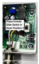
The **Phase Switch** is an internal slide switch that allows you to invert the phase of your signal, so you can perfectly match any additional pickups you might use with your instrument in a multi-system setup. This can also be used to help to increase gain before feedback in difficult monitoring situations.
